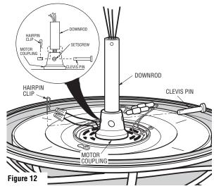
**23.** Install the setscrew (supplied) in the motor coupling and tighten using the 5/32" setscrew wrench (supplied) (Figure 13).
